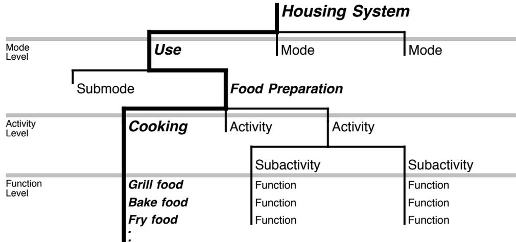
Figure 1. A three-level, top-down analysis is used to find **Functions** that cover the requirements of a system. The result is a **Function Structure**.
