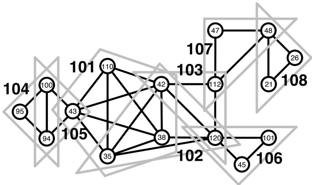
Figure 5. The VTCON program finds clusters of Functions that are highly interlinked. Cluster notation denotes both level and cluster number (i.e., 104 is level 1 cluster 4).
